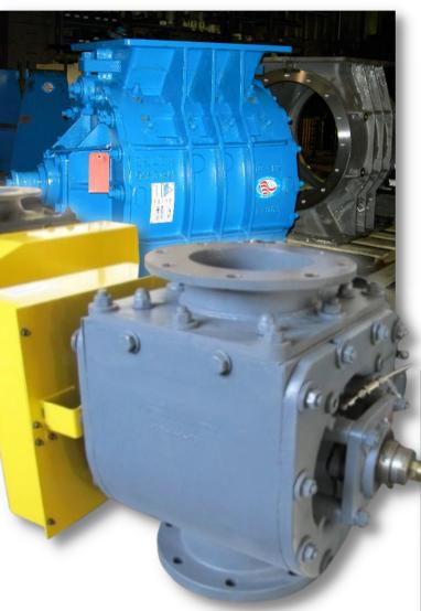
Other valves typically feature a surface hardening that wears away to expose a softer metal base. Once worn these types of valves are often thrown away.
